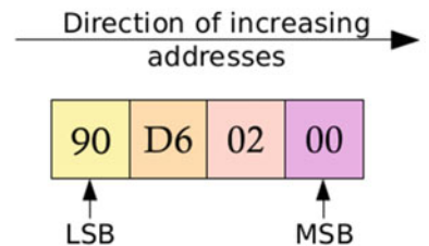
Figure 5-3. A four-byte integer's internal order is independent of the stack direction
