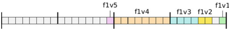
Figure 5-16. A new char variable is added to function f1 after the last local variable
