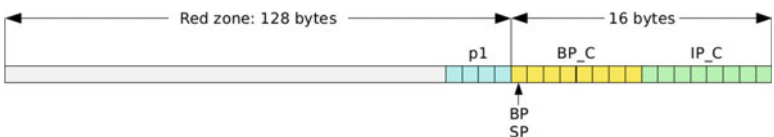
Figure 5-19. The red zone of the stack is used as a private area for storing data
