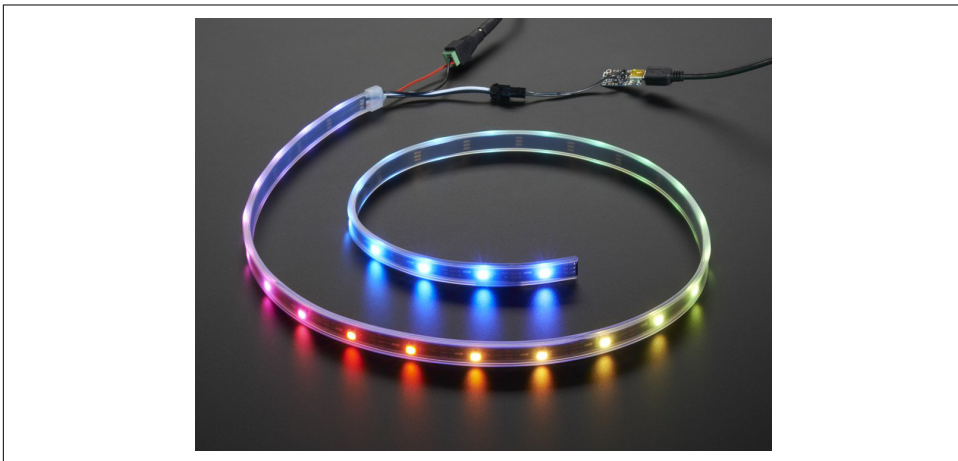
Figure 7-2. A strip of NeoPixels. Also available as rings, flexible boards, and sticks.
