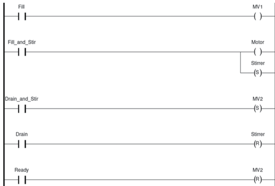
Figure 9.25 Program code based on the state flags
