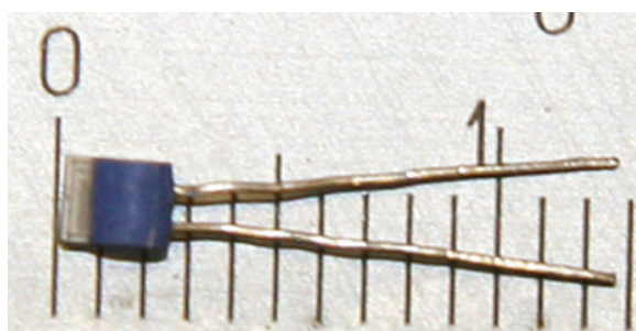
Figure 3.11 Simple sensor—PT100 (thin-film RTD)
