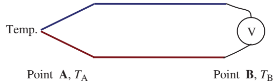
Figure 3.9 Principle of the thermocouple
