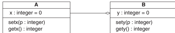
Figure D.10 Aggregation—an object of class B contains an object of class A
