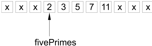
FIGURE 11.1: A pointer to a memory location containing an array of the first five primes.
