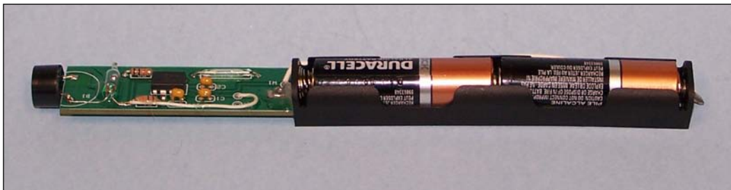
PCB and battery assembly
