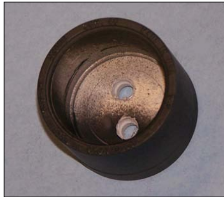
Cap showing drilled holes
