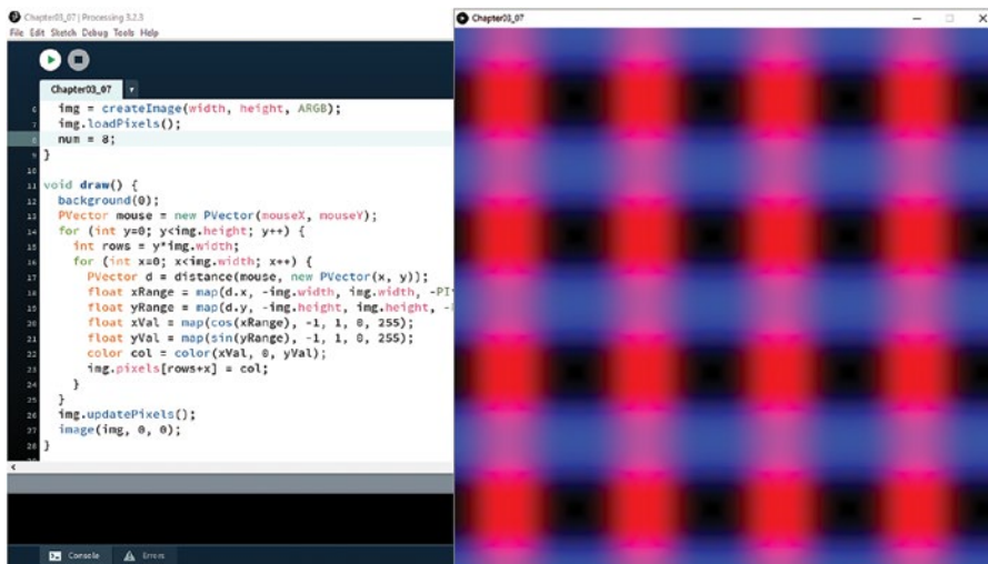
Figure 3-12. Color change with trigonometric functions
