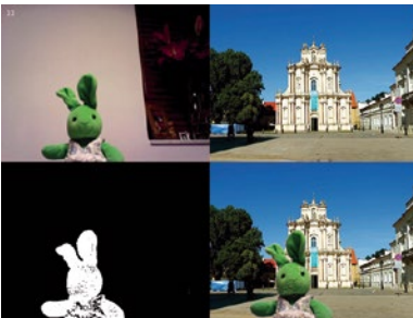
Figure 6-9. Background subtraction and foreground extraction
