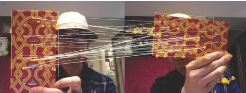
Figure 7-12. Key point matching with a selection rectangle
