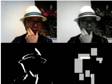
Figure 6-7. Simple tracking with frame differencing
