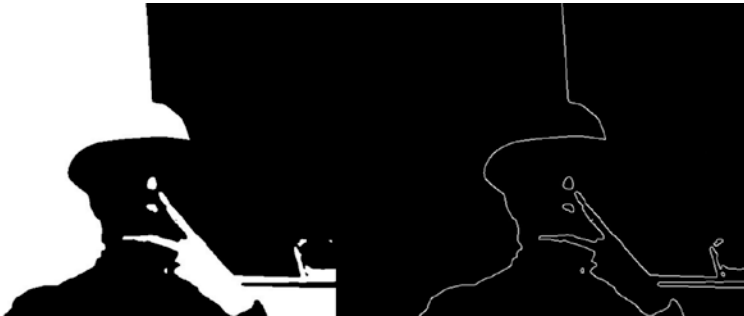
Figure 5-9. Canny edge detection with black-and-white image
