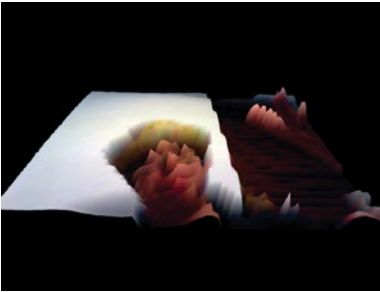
Figure 4-23. 3D effect with brightness as depth
