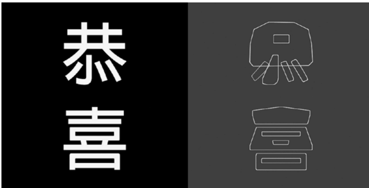
Figure 5-22. Convex hull processing in OpenCV
