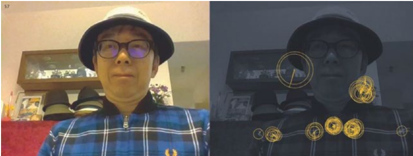
Figure 7-8. Feature detection in features2d
