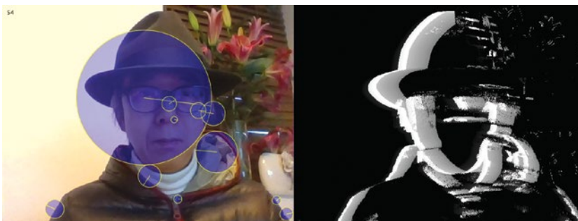
Figure 6-19. Segment motion demonstration
