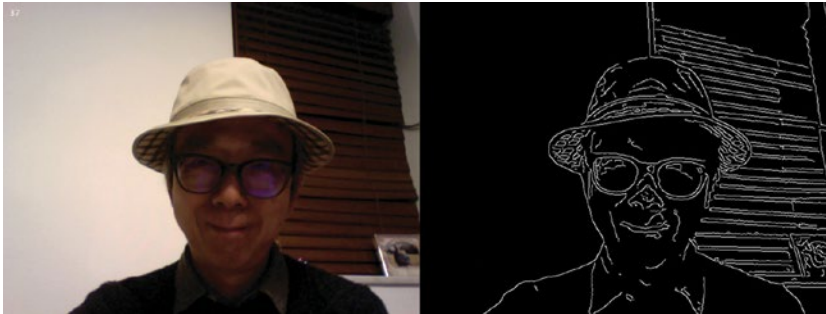
Figure 5-8. Canny edge detection
