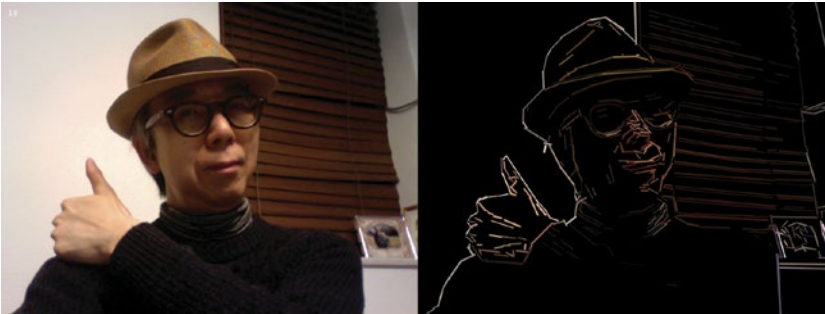
Figure 5-13. Line detection with the OpenCV LineSegmentDetector
