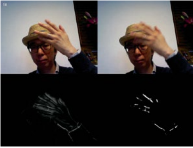
Figure 6-6. Difference between two frames in Processing
