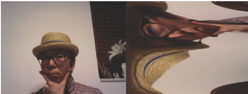
Figure 4-15. Linear to polar transform
