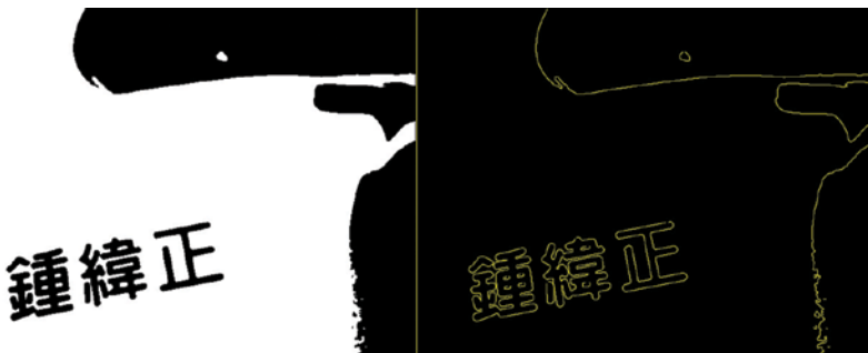
Figure 5-17. Contours processing with threshold image
