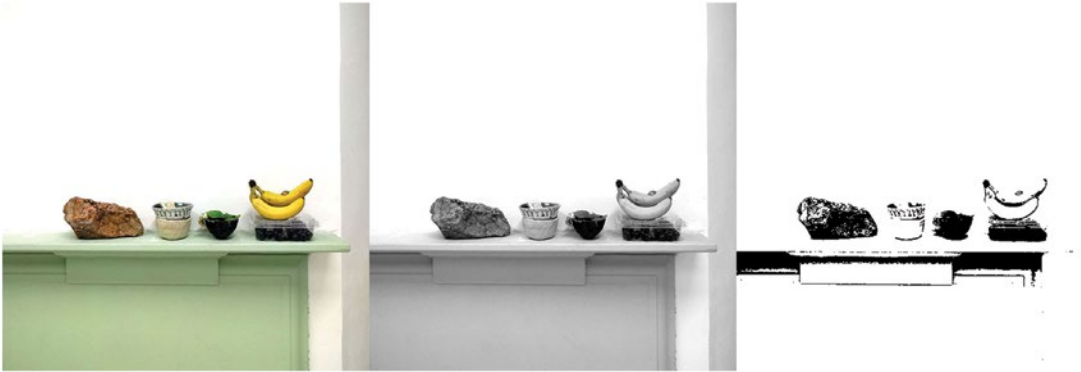
Figure 5-2. Black-and-white image conversion with thresholding
