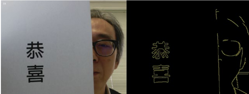
Figure 5-18. Contours processing with the RETR_EXTERNAL option
