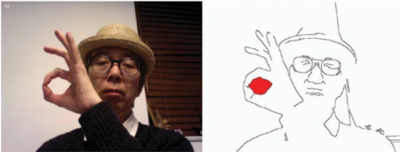
Figure 5-24. Testing whether a point is inside a contour with pointPolygonTest
