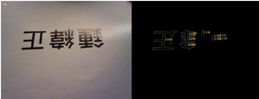
Figure 5-29. Shape-matching test with upside-down characters
