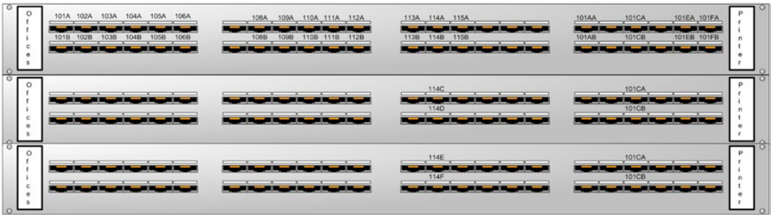
Figure 4-5. Patch panel sequential labeling scheme
