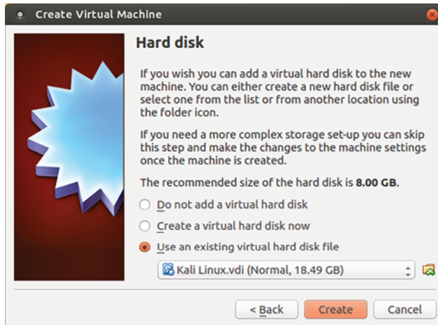
Figure 2.8 The Hard Disk screen. Note how, in this case, the non-default Use an Existing Virtual Hard Disk File radio button is selected.
